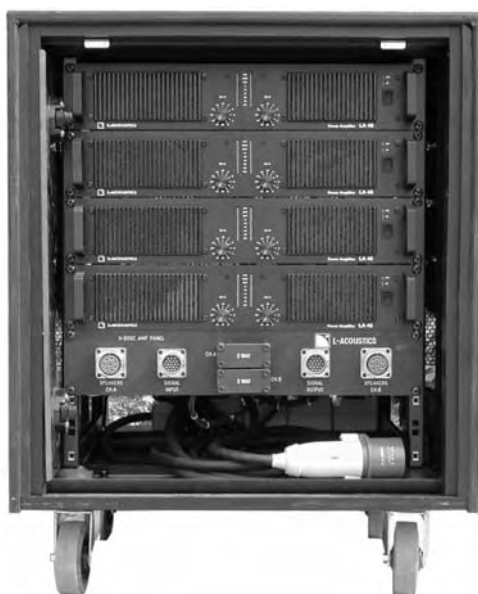
Figure 26: L-ACOUSTICS Amplifier Rack RK124a loaded with 4 x L-ACOUSTICS LA48a amplifiers
