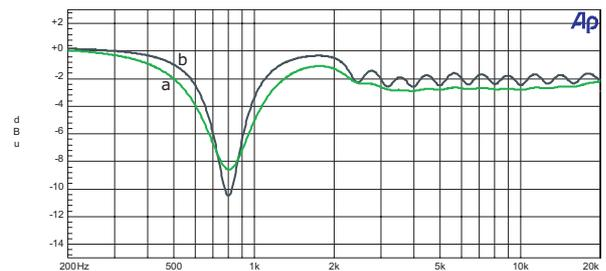
The ability to overlap the notch filters, both with each other and with the graphic EQ bands, allows very deep notches to be created. The adjacent trace shows the responses of a single notch filter, two overlapped notch filters (a) and two notch filters overlapped with an EQ band (b), each resulting in greater attenuation (c). Nearly 45 dB of attenuation is possible when using the notch filters in conjunction with the EQ bands.
