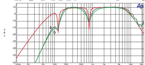
A Symmetrical-Q equaliser lacking the additional filters cannot produce a high pass filter response using just its faders, either with a narrow or wide response (a and b traces). The user may assume that subsonic frequencies are being attenuated by cutting the bottom faders but the graph shows that this is not the case.
