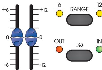
The range of the faders on each channel is switchable using that channel's RANGE switch between  $\pm 6$ dB and  $\pm 12$ dB. The current setting is indicated by the '6' and '12' LEDs above the range switch.
