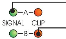
**Signal** - The signal LED shows incoming signal to the unit and is Pre EQ (but post gain control).
