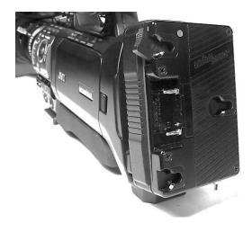
The Camera described in this section is the GY-HM790U equipped with the Anton Bauer battery mount. The GY-HM790E is equipped with the IDX "V-Mount" Battery mount.
