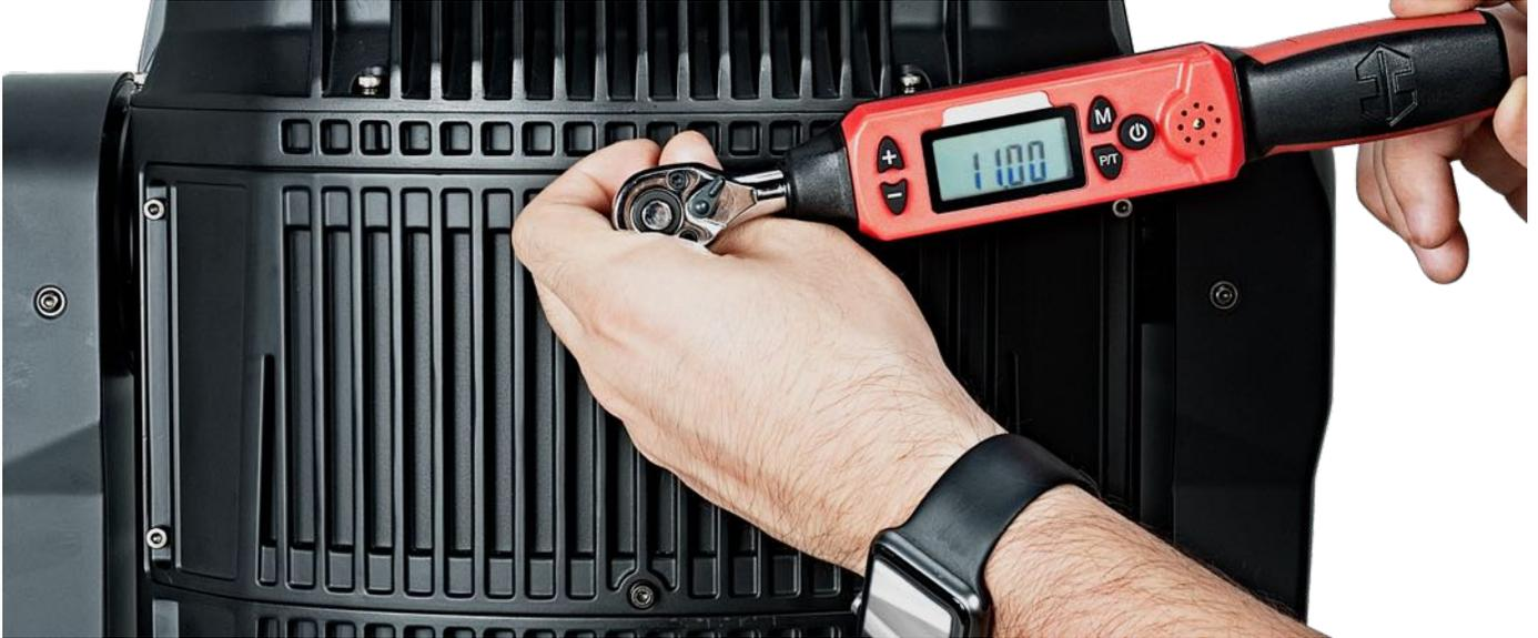
The (12x) hex-head screws holding the panels **MUST** be tightened with a torque wrench (not included). **TORQUE SETTING = 11 lbf-in. (12.7kgf-cm) \***
