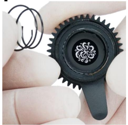
12. Carefully remove retaining spring.
