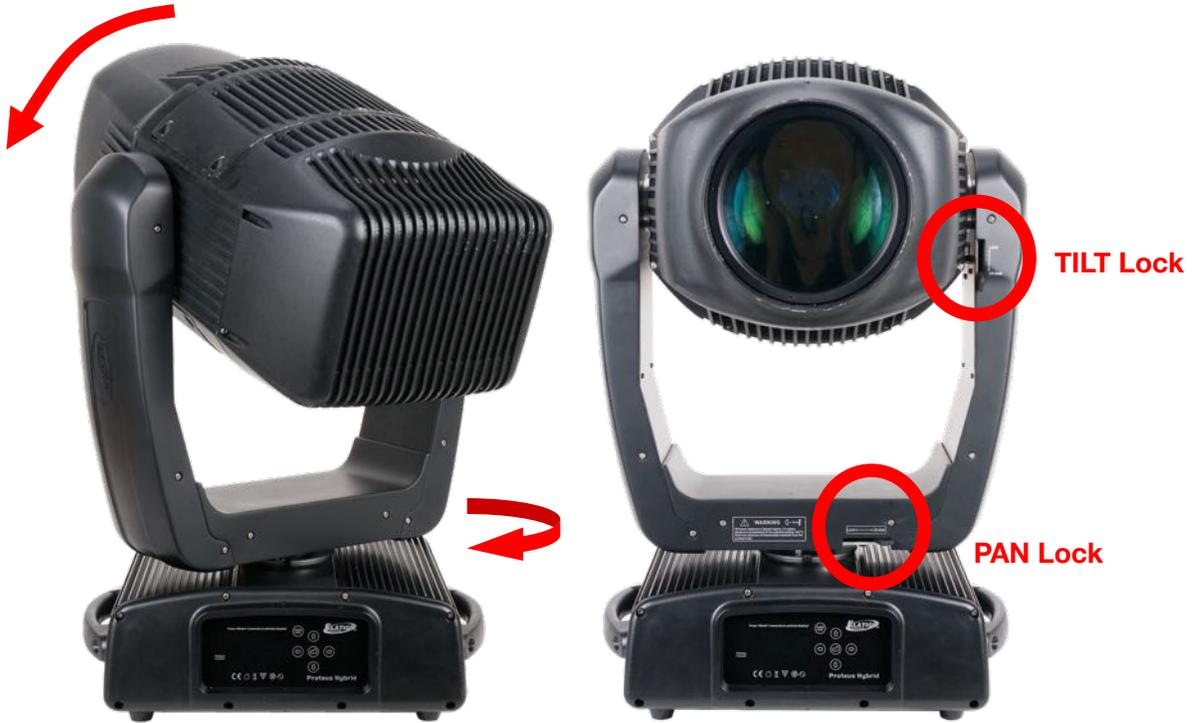
2. Place head in a right-angle horizontal position and engage both the **PAN** and **TILT** locks for added stability while replacing the lamp.
