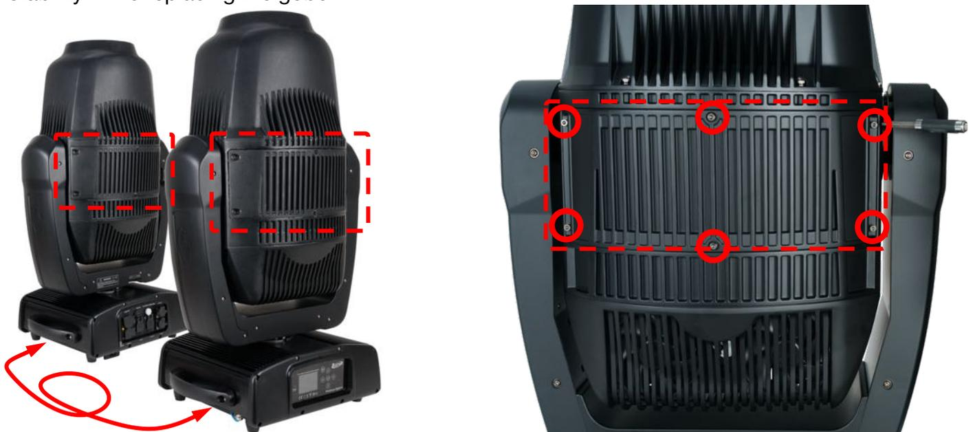
3. Remove (12x) 3mm hex-head screws (6x per panel) to remove both center panels.
