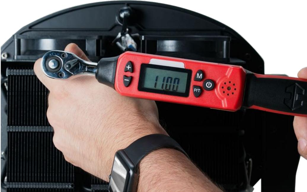
The (4x) hex-head screws holding the heatsink module **MUST** be tightened with a torque wrench (not included). **TORQUE SETTING = 11 lbf-in. (12.7kgf-cm) \***
