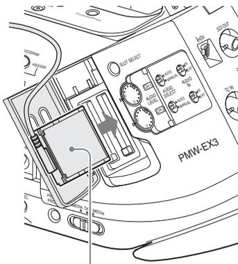
Insert so that the cable extends upward.
