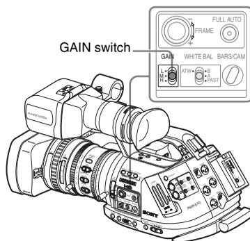
The gain value at each of the switch positions are set at the factory are as follows:
