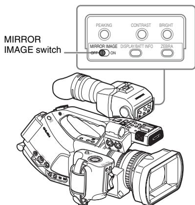
When the camcorder is in Media mode, the picture is also inverted both vertically and horizontally. In Camera mode, the picture is inverted only vertically, while it is also inverted horizontally for Rec Review (page 73).
