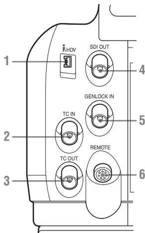
1. **i.LINK (HDV)** connector (4-pin, S400 conforming to IEEE1394) (*page 136*)
