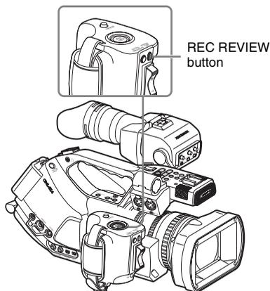
After recording is finished, press the **REC REVIEW** button or the assignable button to which you assigned the Rec Review function.
