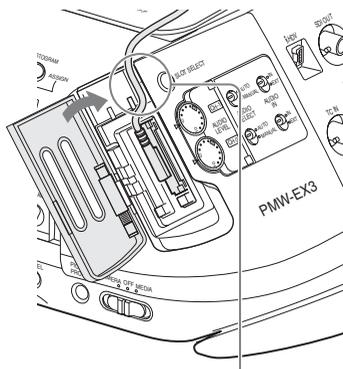
Pass through the cable guide slot.
