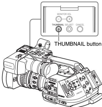
The thumbnail screen changes such that it contains only the clips marked OK among the clips on the current memory card. To return to the thumbnail screen with all the clips, press the THUMBNAIL button again.
