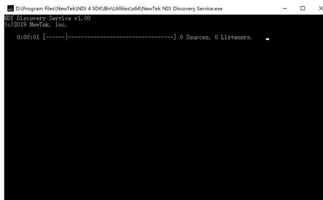
The NDI encoder configures the IP address of the receiving end in the discovery server, and the NDI will be registered to the server. It is recommended that the receiver address be configured as a static IP address to prevent the loss of NDI connections due to IP reassignment.
