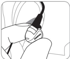
Insert the earphones so they form a tight seal. The fit of the earphone can greatly affect sound quality.
