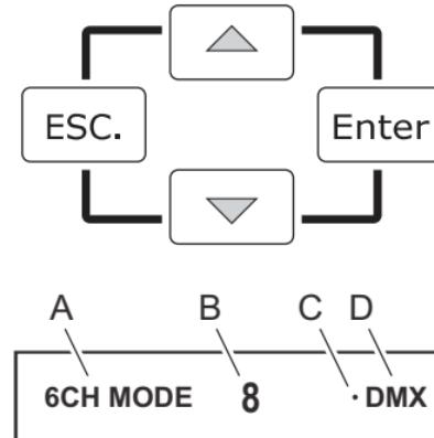
The fixture is set by default to be controlled in DMX mode.
