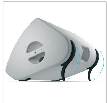
► Built-in risers offer two stage angles:  $35^\circ$  or  $55^\circ$  with regard to vertical to accommodate short or long throw stage monitoring applications.
