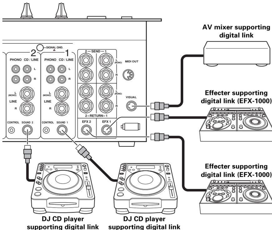
By connecting a single dedicated cable (digital link cable), exchange of audio signals and control signals can be performed digitally (The connection of audio cables or control cables is unneeded).
